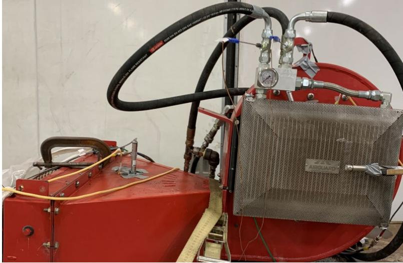
**Figure 1.** Airguard BPS mounted to a Morris air cart fan.
