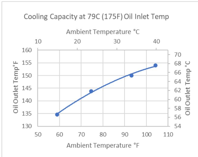
**Figure 3.** Airguard BPS hydraulic oil cooling capacity (at 79°C [175°F] oil inlet temp).
