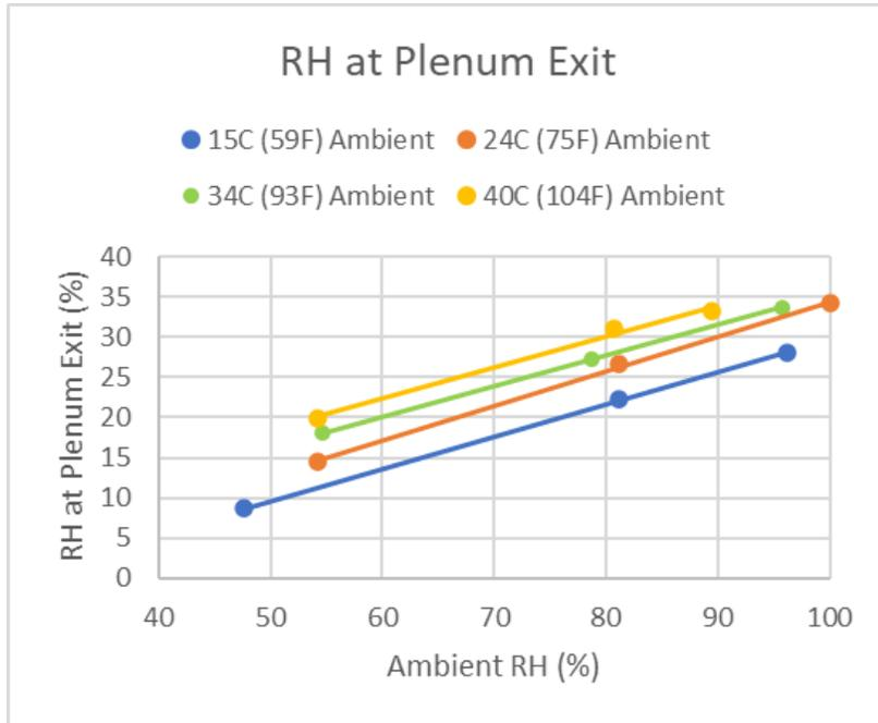
**Figure 2.** Relative humidity reduction measured at the plenum exit.
