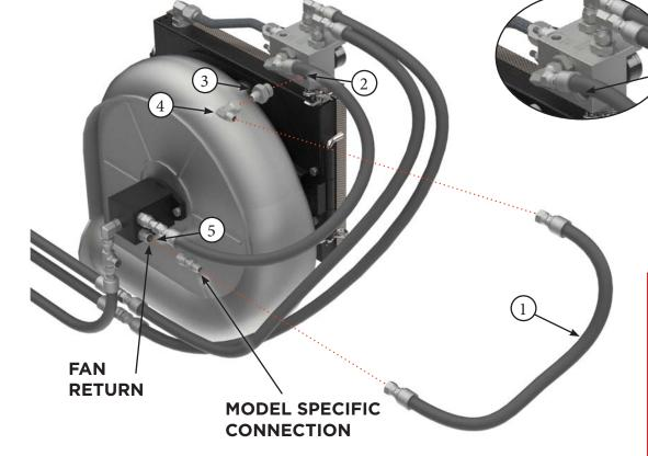
PARTS LIST Part # Description Item BPS 1/2" Hydraulic Hose - 60" 7267 1 2 "FAN RETURN" Port - BP System Manifold \_ \_ 3 9096 Fiting - Straight - 1/2" JIC Male - 3/4" ORB Male
