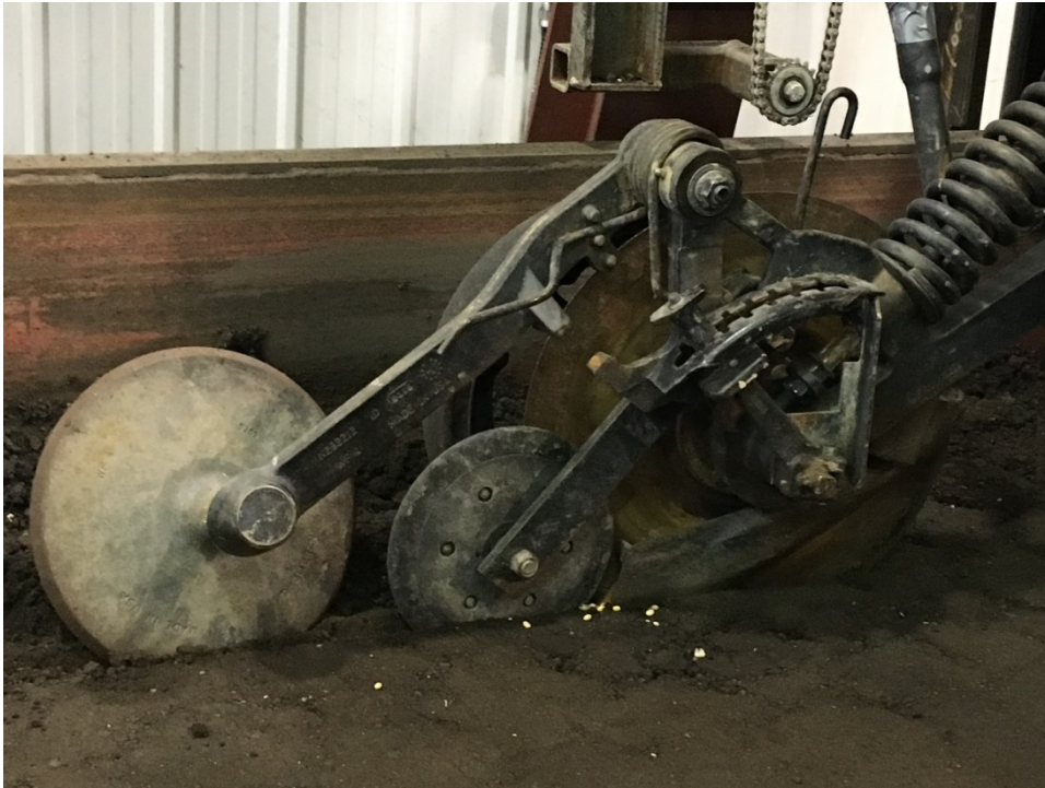
Figure 1. The terramechanics soil bin used for planting soybeans with a disc opener.
