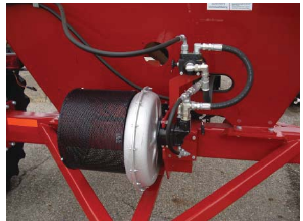
The blower and associated hydraulics
